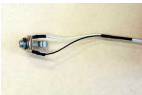
Pilot Headphone jack soldered and heatshrink
