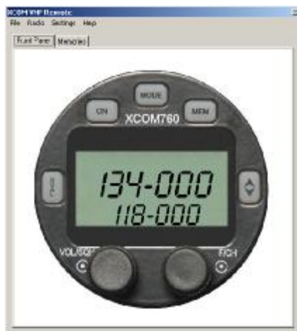
The XCOM Front panel screen, controlling all the operations of the XCOM VHF radio remotely.
